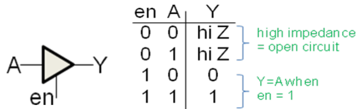
Tri-state buffer gate symbol and truth table.
