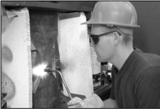
Keith Kowalkowski, graduate research assistant, applies heat to a damaged specimen of steel, one of 90 such specimens that he will test.
