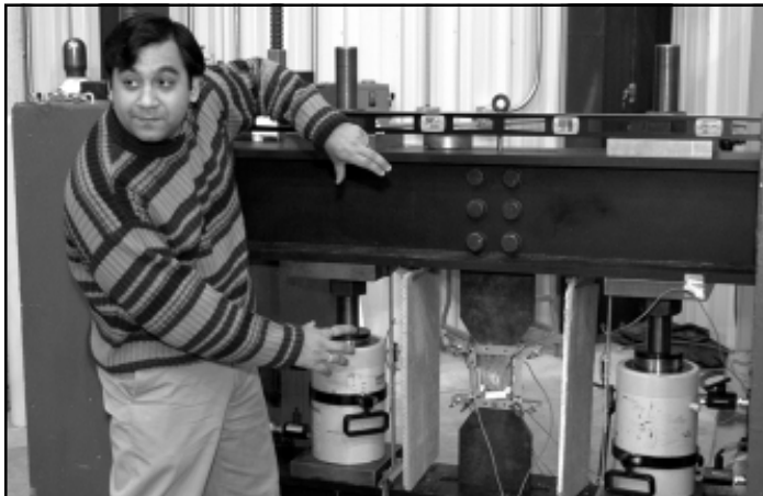
Dr. Amit Varma explains the laboratory setup for small-scale tests on the effects of heat-straightening.
