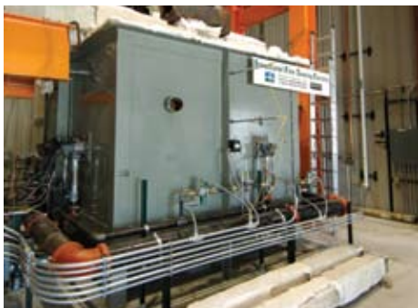
The furnace in the facility generates heat up to 2,200 degrees Fahrenheit.
