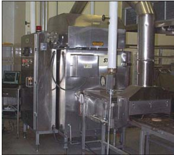
A pilot-scale, moist-air impingement oven.
