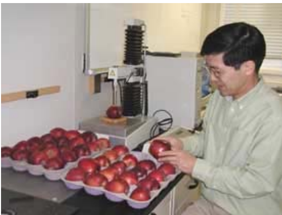
Dr. Lu is measuring firmness using a texture analyzer
