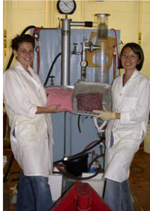
Nutrition graduate student Katie Barrett and BE Graduate Student Kathy Lai holding spray-dried powder (final product) and grape pomace (source). Behind them is a bench-scale vacuum evaporator used to concentrate liquid extracts from grape pomace, culled blueberries, and culled onions.
