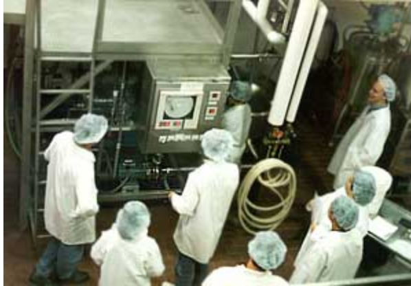
Falling film evaporator for concentrating fluid products. (Dr. Marks on far right)
