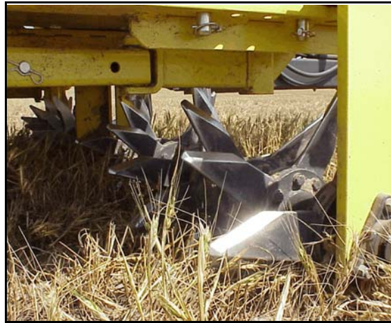
A rolling-tine harrow fractures the soil and improves infiltration with little soil inversion or loss of protective residue.
