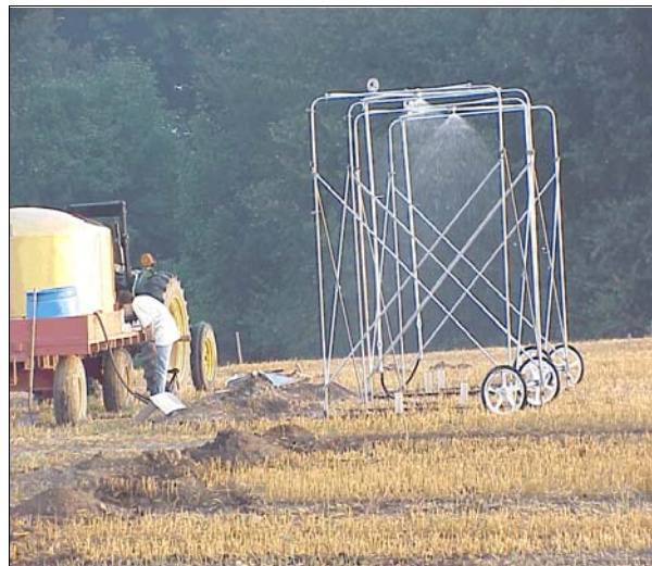
Portable rainfall simulators were used to simulate rainfall events on days 3, 10 and 21 after manure application.
