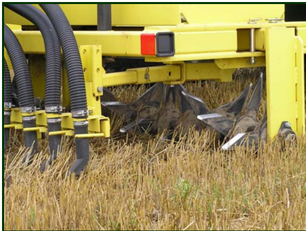
The rolling-tine aerator loosened and fractured the soil while the drop tubes flooded the loosened soil with seed-laden swine slurry.
