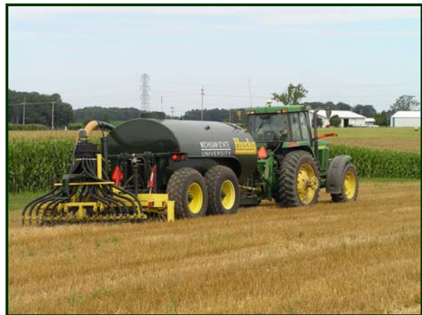
The seeding process incorporated low-disturbance aeration tillage, manure application, and the seeding of cover crops in one efficient operation.
