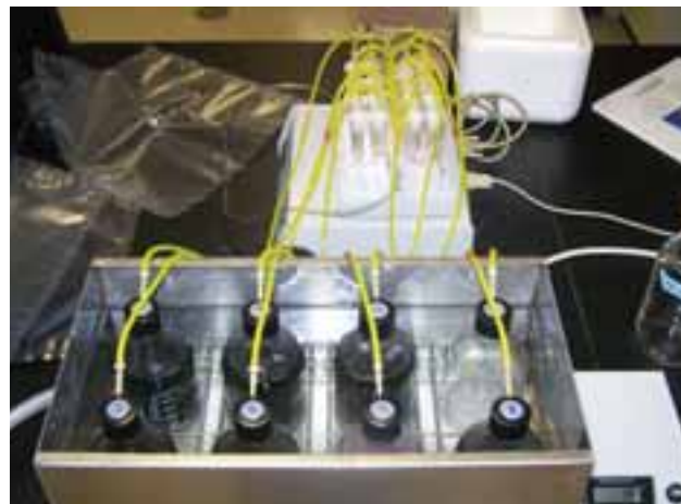
An anaerobic respirometer is used to provide biogas potential assays.
