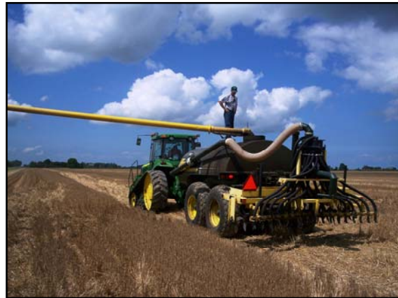
Fig. 1. Volatile ammonia losses following aeration tillage with sub-surface slurry deposition was compared with losses from surface spreading and surface spreading with rapid incorporation.
